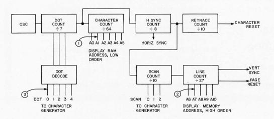
Figure 1: Block diagram of a television display. This version is very similar to the display described by C W Gantt in June 1976 BYTE, page 18. The points indicated by circled numbers are used as described in the text to generate the various test patterns shown in photos 2, 3, 4 and 6.
