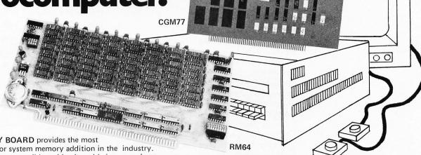
THE RM64 MEMORY BOARD provides the most cost effective means for system memory addition in the industry. The board is S-100 bus compatible making it usable in over a dozen different microcomputer systems including ALTAIR and IMSAI.
