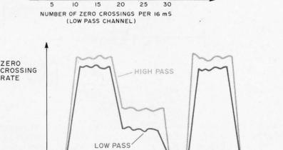
Figure 4a: A plot of the word "SIX" showing the zero crossing rate as a function of time. The word is shown split into its four phonemes. In this case, the signal is first processed through two bandpass filters. The number of zero crossings is then determined by the computer. Results for both filters are shown. As the graph indicates, there is a very short period of silence during the pronunciation of the KX phoneme which can be verified by slowly pronouncing the word "six."
