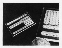
The Machine and Control Division of Interrotech, POB 128, Farmington ME 04938, has announced a new drafting template for \$8.95 to be used in designing "tapeless" printed circuit board layouts using ink pens, or pencils. The template produces pin layouts of dual in line integrated circuits that are twice actual size. The template has a versatile pattern that includes all the popular sizes up to 40 pin packages.
