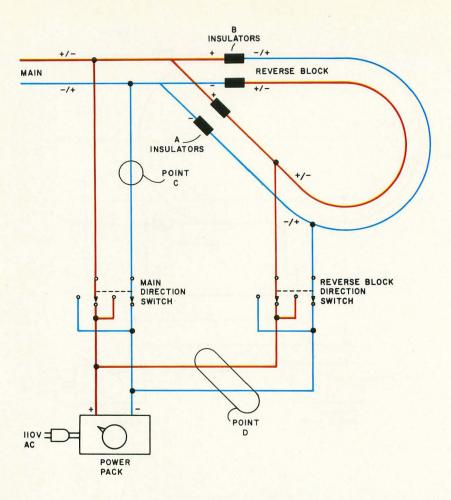
Figure 4: Using insulators on both the positive and negative tracks a block is created that is totally isolated from the main track. Using a separate power pack will allow the train to run through the block, turn around, and return to the main track.
