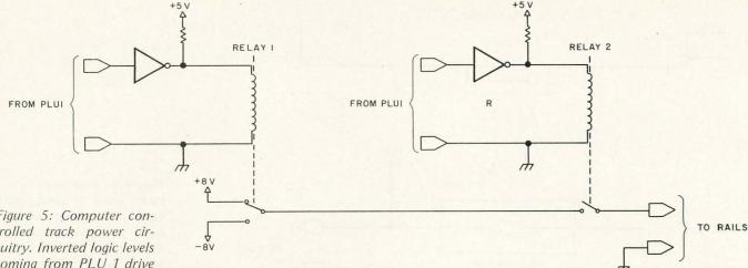
Figure 5: Computer controlled track power circuitry. Inverted logic levels coming from PLU 1 drive two types of relays. The first type (represented by relay 1 in this illustration) chooses the polarity of the voltage going to the track, while the second type (relay 2 here) applies power to the track. Only certain strategic areas of the track require polarity switching.
