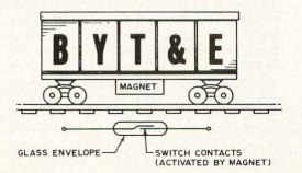
Figure 6: This is a magnetic reed switch which can be used as a marker along the track. The switch consists of two contacts that are enclosed within a glass envelope. The two metal contacts are activated magnetically when a car with a magnet attached passes over.
