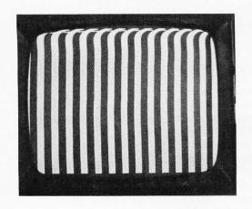
Photo 2: Exploring the circuit with the probing alligator clip produces various interesting signals. Here the clip looks at address bit 1, point 1 on figure 1. This signal changes state every other character position, giving vertical bars two character widths wide. Note the distortion at the top of the image, not normally seen due to blanking of the display.
