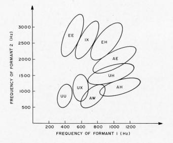
Figure 2: Vowel phonemes on the formant plane. "Formants" are the natural resonant frequencies of the vocal tract. These resonances are similar to the resonant vibrations of organ pipes or the characteristic sound of an empty bottle when air is blown across it. The three most prominent formants are centered around 500, 1500 and 2500 Hz, but they vary with changes in position of the tonque, lips and mouth.
