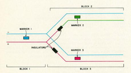
Figure 8a: An example of a marker being between two blocks. In this type of array the computer must only determine whether the train will go into block 2 or 3.
