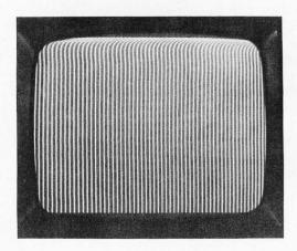
Photo 5: A garbage display field, obtained by the application of power to the memory. Each chip has a preferred start-up value, so this pattern tends to be the same whenever one turns on the display. In this picture, blanking
