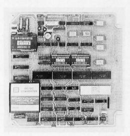
Signal Laboratories Inc, 202 N State College Blvd, Orange CA 92668, is making available a new analog IO card. With this board, intended for use with the Zilog Z-80 development systems, the engineer or scientist can monitor up to 16 analog channels in real time.
